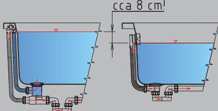
Automatic pop-up waste MAAX is suitable for any Polysan bathtub. It enables you to fill bathtub almost to the edge. You do not really realise missing overflow. UP&DOWN waste is controlled just by plug pushing.
